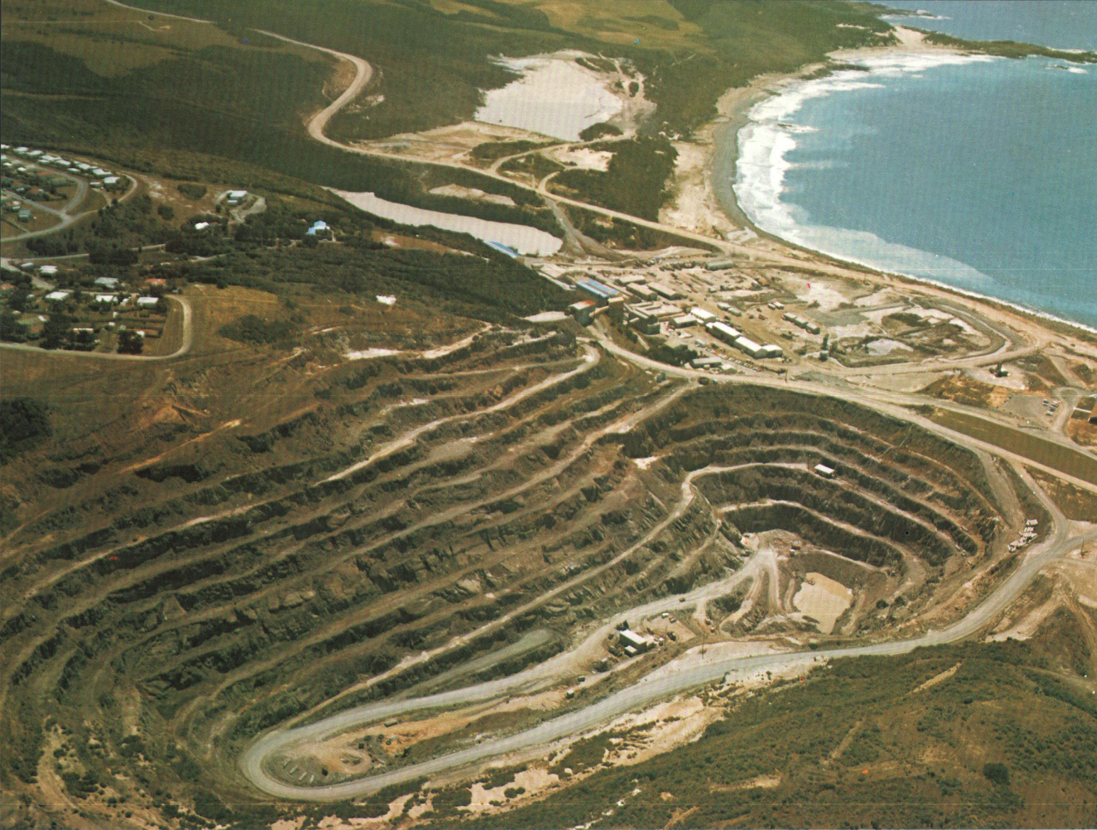
King Island Scheelite's open cut mine which closed in 1974. The Dolphin Mine portal is at the bottom of the pit; the works and part of the township of Grassy can also be seen. (see Ch. 8)
