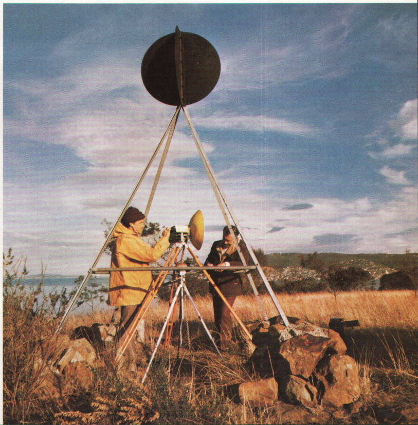
Electronic distance measuring from a trigonometrical station
